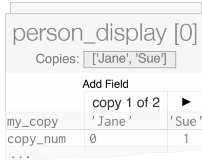
Figure 4.15 An object with multiple copies; copies is set to ['Jane', 'Sue']. Every copy has two properties: my_copy , which is set to that copy's item (here, either 'Jane' or 'Sue') and copy_num , which is set to that copy's index. Here, we are looking at the first copy (index 0).
