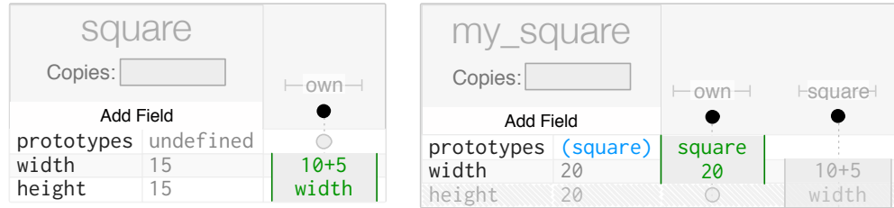
Figure 4.13 InterState uses a prototype-instance inheritance model with multiple inheritance. Prototypes are simply specified in the prototypes property. Here, my_square inherits from square . Because my_square does not define a value for height , it inherits the definition of square.height , as indicated by the greyed out text in the columns on the right. Note that my_square inherits the definition of height , not the value. Thus, the width property of my_square evaluates to a different value (20) than the width of square (15).
