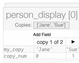
Figure 5: An object with multiple copies; copies is set to ['Jane', 'Sue']. Every copy has two properties: my_copy , which is set to that copy’s item (here, either 'Jane' or 'Sue') and copy_num , which is set to that copy’s index. Here, we are looking at the first copy.
