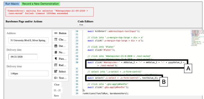
Figure 3. An error is shown when a particular CSS selector does not exist on the page.
