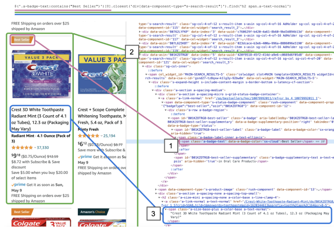
Fig. 1. To query the Amazon DOM for the first “Best Seller” and get the item’s name, (1) query for the first “Best Seller” label, (2) query for its ancestor that represents the full item, and then (3) query for the item name.
